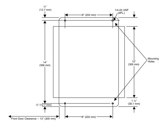
Figure 3-1: LTC-MAP 2130 Monitor Mounting Dimensions
